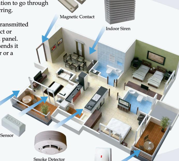
• The system allows you to remotely call in to arm and disarm from wherever you are. Through configuration at a predetermined time, the system can initiate auto arming
