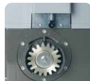
Integrated limit-switch in opening and closing
